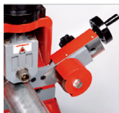
Large tube stabilizer up to 12"
